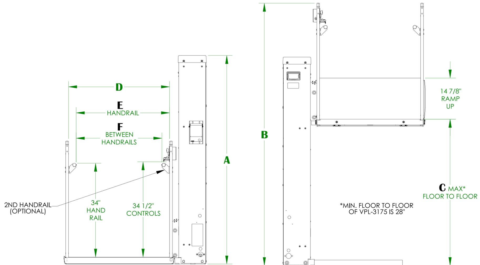
NOTES: 1) ACCESS RAMP CAN BE MOUNTED ON EITHER SIDE OF THE PLATFORM
