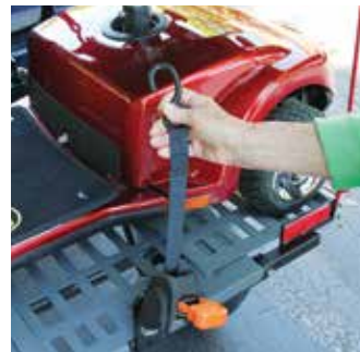
Self-tensioning retractable securement belts.
