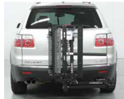
HTP Mid Wheel Drive (MWD) accommodates MWD powerchairs with 10 in and 14 in wheels.
