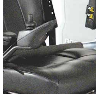
Hold-Tite arm securement for powerchairs.
